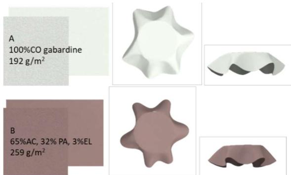
Figure 3: Simulated fabrics with different fabric properties.
