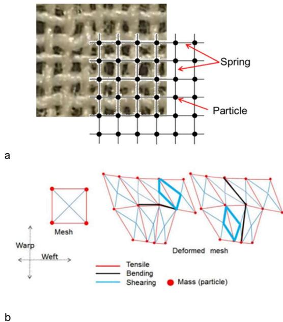
Figure 7: Translation of physical fabric parameters into a particle mesh [28].
