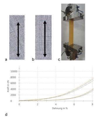
Figure 10: Tensile and shear elongation in (a) warp and (b) bias direction (c) ZwickRoell tensile test device and (d) elongation/force curve.
