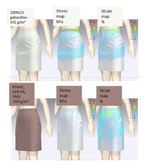
Figure 8: Simulated results with stress and strain maps for a skirt in different fabrics.
